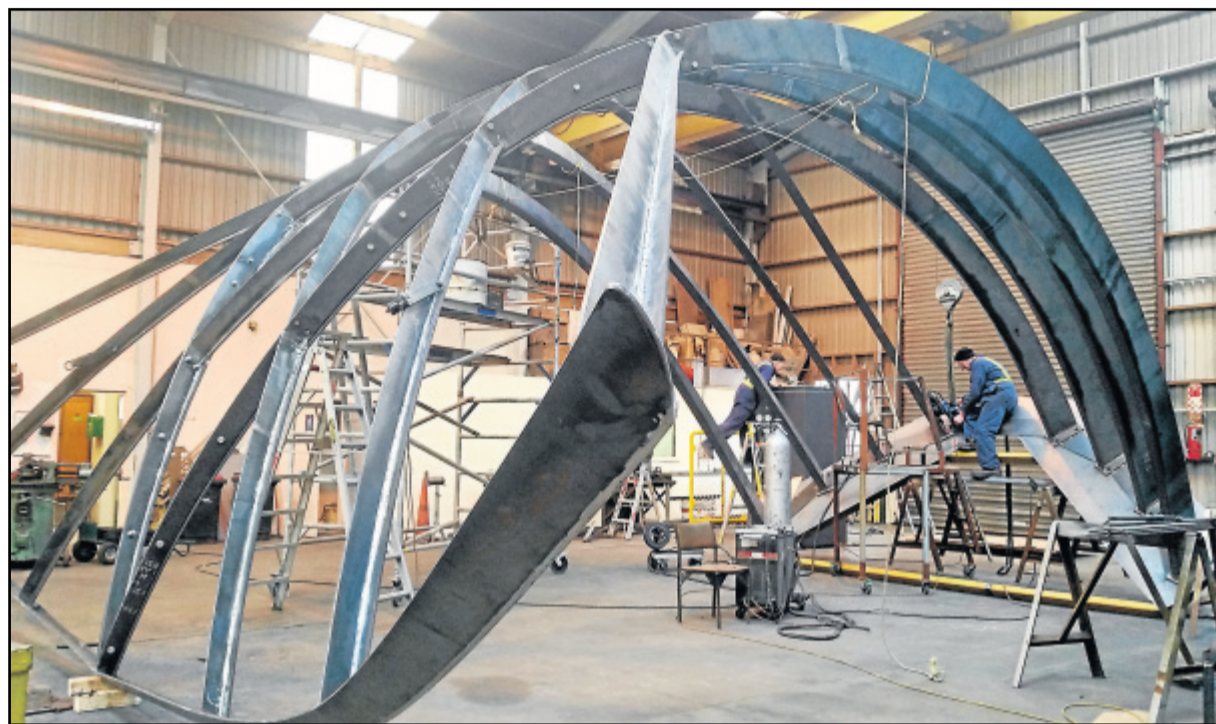
The sculpture, near the end of the fabrication phase, in a prone position for access. It will soon make its way to be painted which will take three weeks followed by installation including lighting and landscaping.
